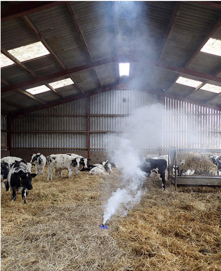
Smoke bombs can be used to demonstrate problems with ventilation in sheds.
